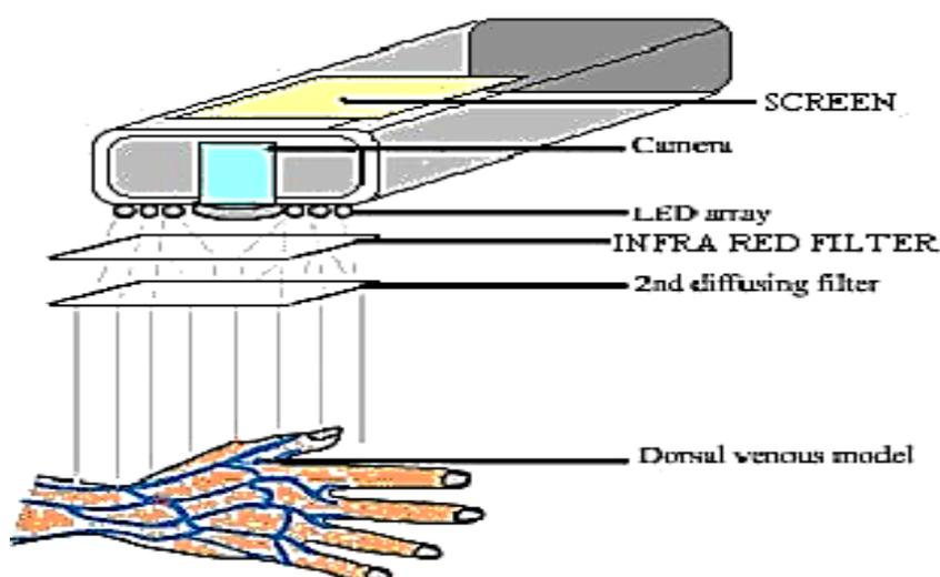
**Fig 1:** Working principle of the model (17).
